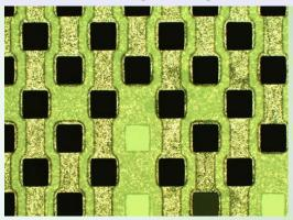
Metallization 2-Probe Circuit
