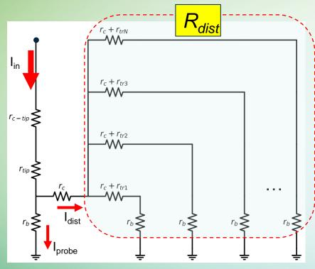
$$R_{dist} = \left(\sum_{n=1}^{N} \frac{1}{r_c + r_{tr(n)} + r_b}\right)^{-1}$$
