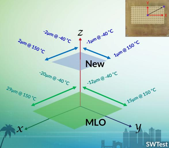
Simulation of thermal expansion at high temperature **New Substrate** MLO Item - 40 40 36.027 Max 28.822 25.219 25.219 21.616 21.616 Pattern 18.014 18.014 14,411 14.411 simulation 10.808 7.2054 7.8584 Ma 3.6027 3.6027 0 Min 0 Min Maximum 25 ~ 40 µm < 5 µm deformation
