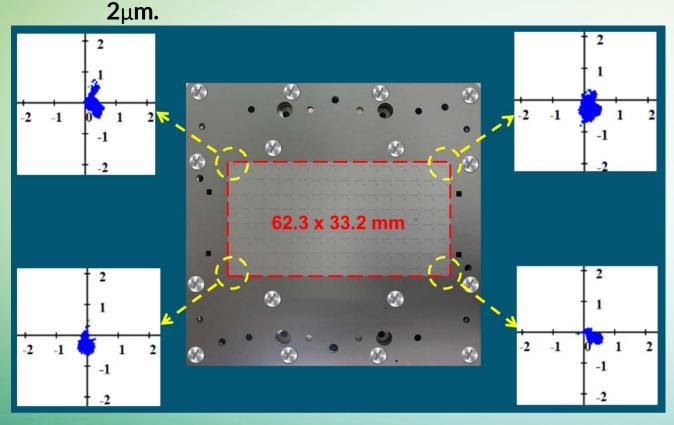
Bottom Left | Bottom Right **Top Left Top Right** Temp. 25°C 4.0 µm 4.5 µm 3.4 µm 3.9 µm 150°C 5.0 µm 5.4 µm 6.5 µm 6.8 µm
